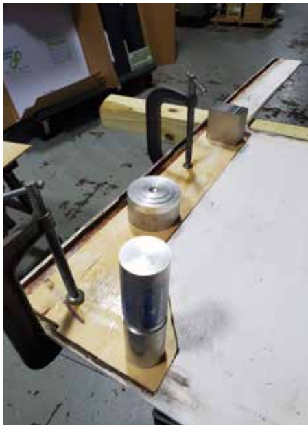
Bonding the new core in place
