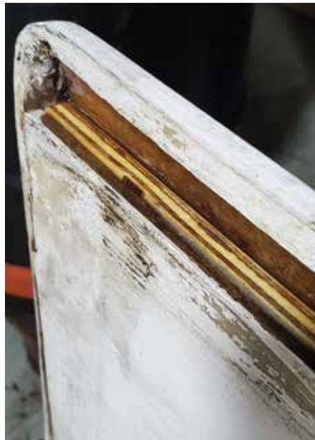
Sealing the edges of the new core
