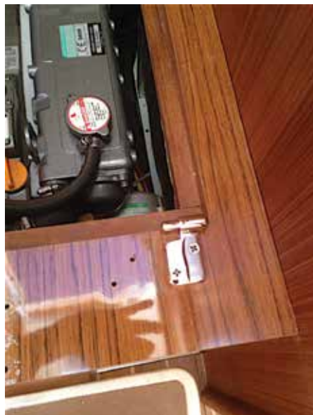
The port side pintle leaf screwed in place – showing the correct fore/aft position axially aligning the pintle structure with the gap.
