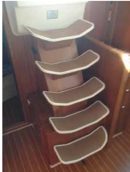
The companionway stair assembly. Note the position of the piano hinge
