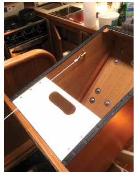
Showing the upper stair assembly tilted forward after the hinge replacement. Note the hand hole I cut in the delrin part – very helpful during the removal procedure.
