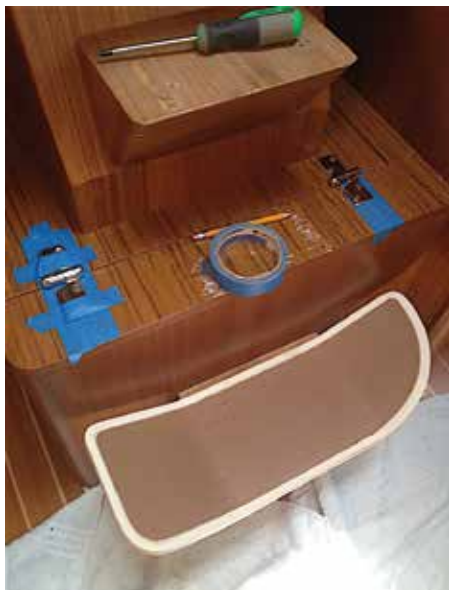
Upper and lower structures returned to normal position. Two "take-apart" hinges positioned and held in place with blue masking tape prior to being screwed in place.
