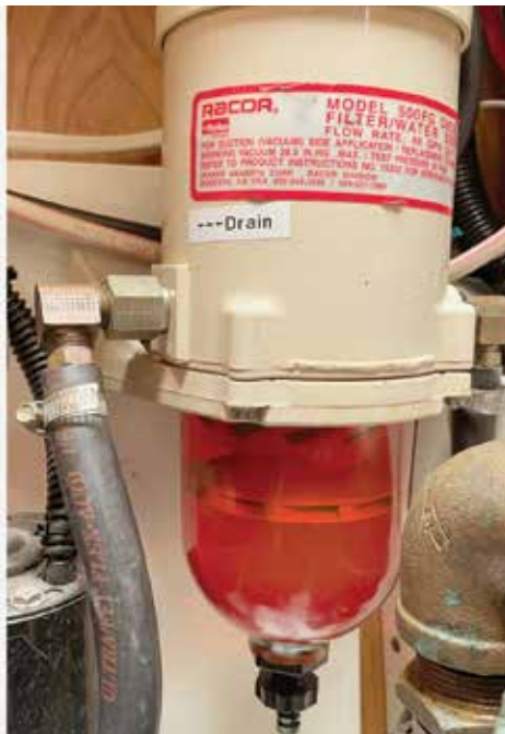
Racor filter showing sediment bowl half full of schmutz from a bad batch of diesel. Before and After. Photos by Joe Rocchio.
