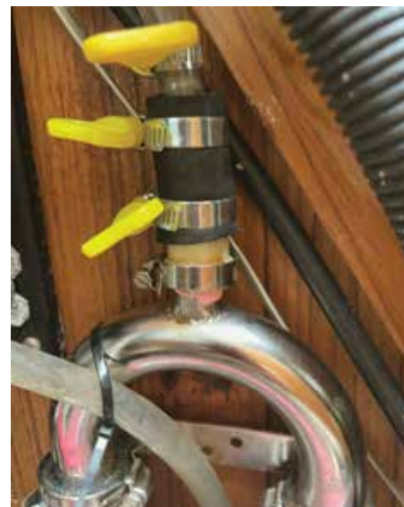
Engine vented loop drip catcher for leaking vacuum break valve. Carries slow drips through a hose from faulty valve to bilge to prevent water damage to engine compartment. Photo by Joe Rocchio.
