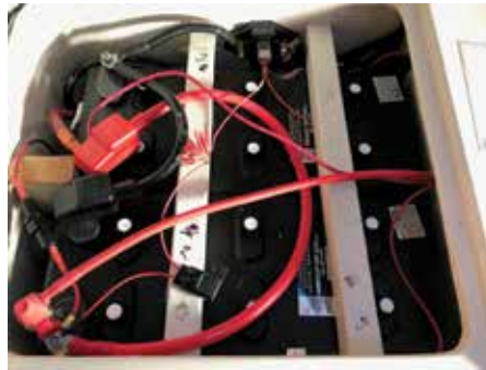
The SG200 shunt is in the back between the two hold down bars. Note battery terminal caps.
