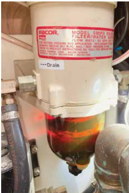
Racor filter showing sediment bowl half full of schmutz from a bad batch of diesel. Before and After. Photos by Joe Rocchio.
