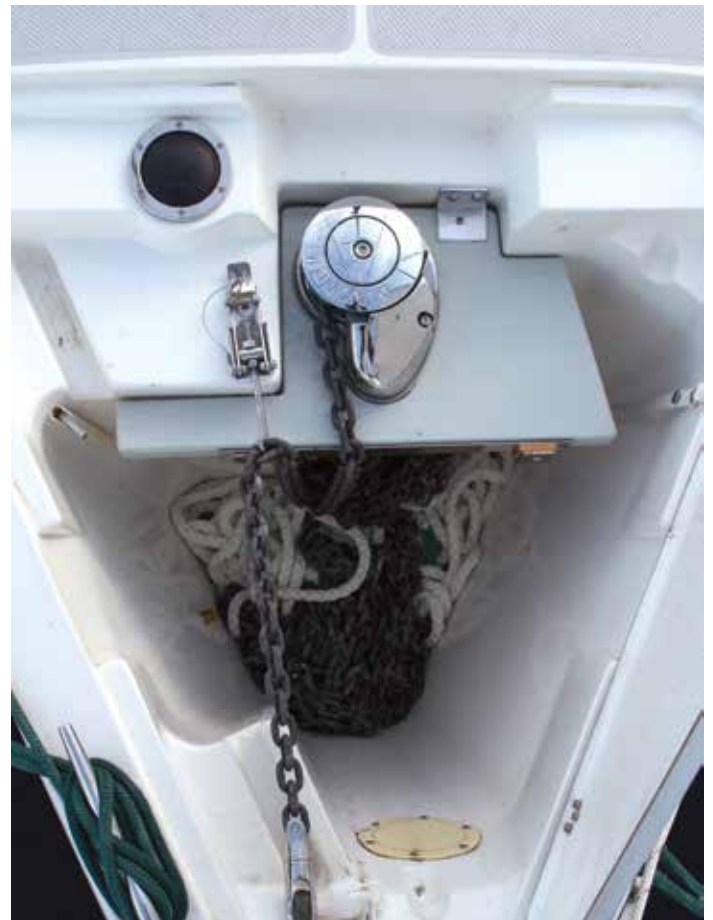
Completed install with rode in place and chain tensioner installed. The bracket to the right of the windlass was added to stop the "bounce" during retrieval.
