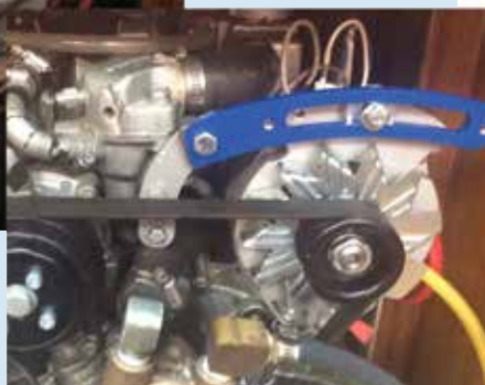
Right image shows the modification to the arm.
