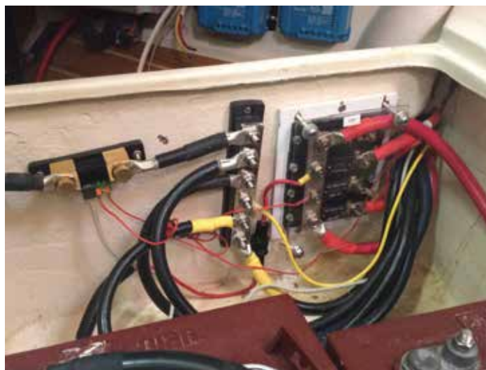
Installation of fuse block and negative bus in battery compartment.
