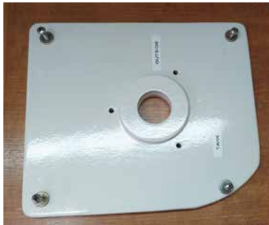
The cover/valve mount was made from a piece of marine plywood.
