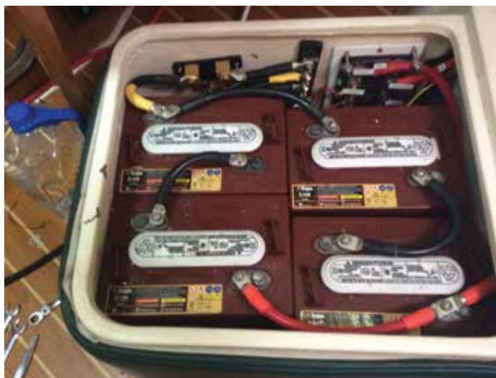
House bank rewired with 4 Trojan golf cart 6 volt batteries.
