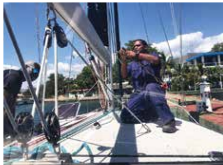
Otto quickly replaced the blown rivets on our boom.
