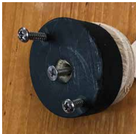
Assembly of fan pedestal for mounting in globe cage
