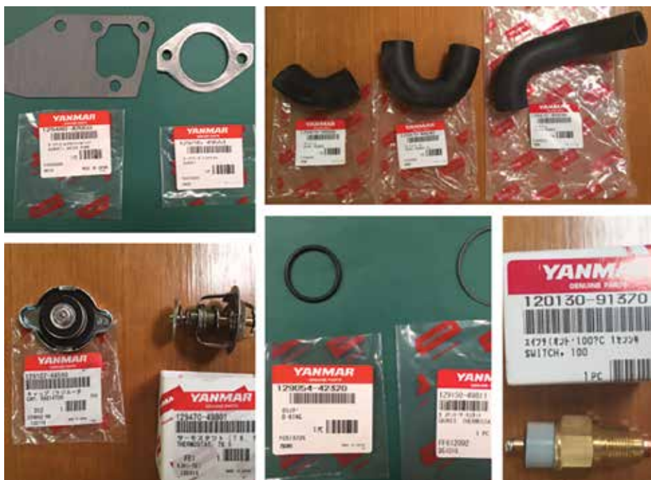
Ancillary parts required for coolant water pump replacement.
