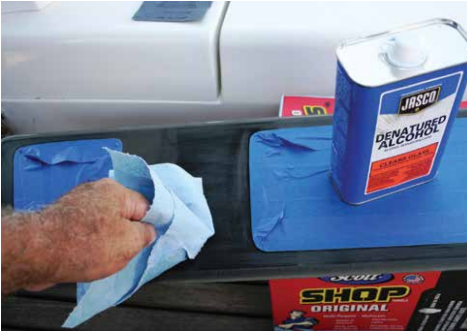
Sanded and Cleaned Lens Mounting Surface
