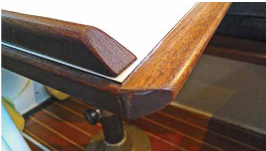
Corner Detail with Old Inboard Fiddle and the New Edge with Teak Oil
