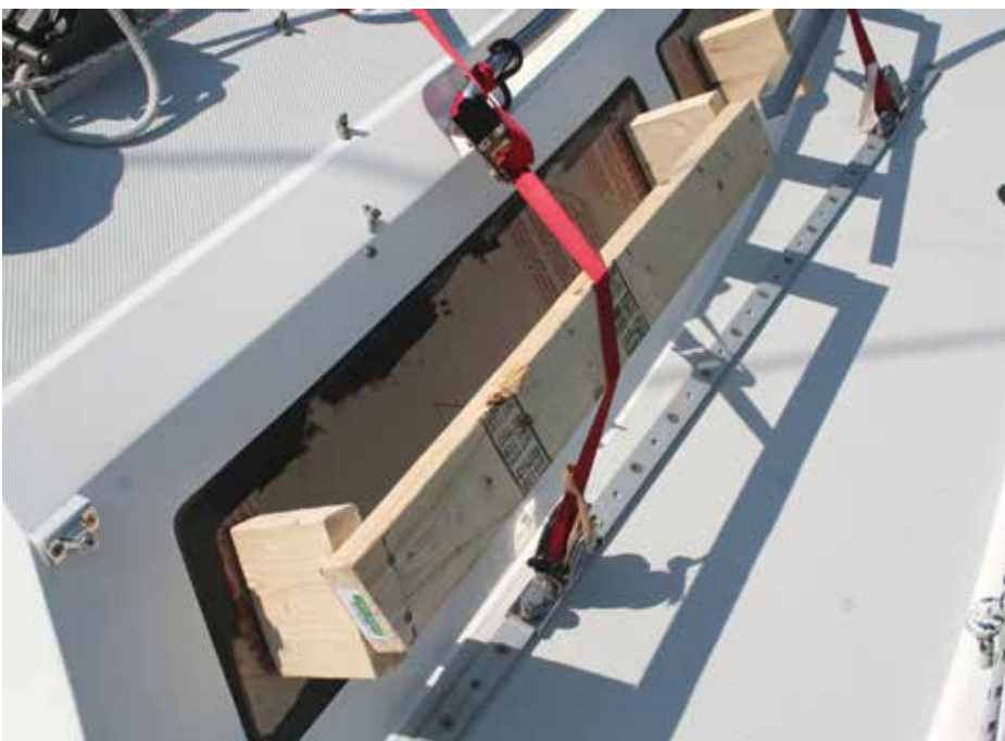
Window Lens Installed, Clamped and Edge Finished
