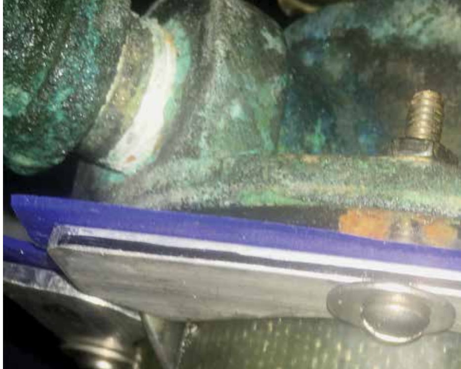
Water strainer brass top and plastic can showing the area of epoxy and fiberglass repair and reinforcement with aluminum strip.
