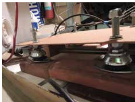
Using a Template of the Beta 20 to Size the New Oak Engine Beds
