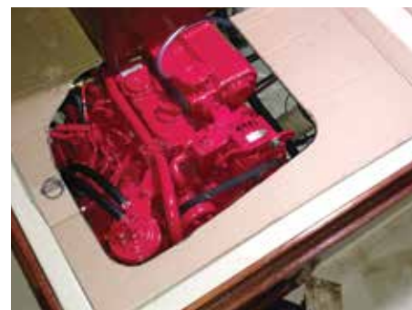
Template to Construct an Engine Compartment Cover With Raised Engine Cutout
