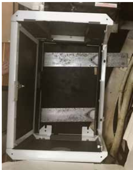
Sound enclosure for M673LD3G test-assembly in compartment. Photo by Joe Rocchio
