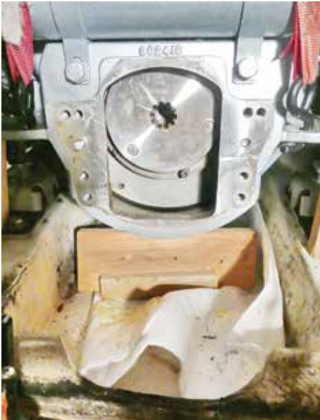
The straps led aft of the heat ex-changer and hooked to the engine mounts
