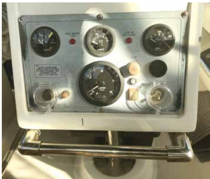
Onward's Cockpit Console and Engine Control Panel with Switch Protection Covers and Telescoping footrest.
