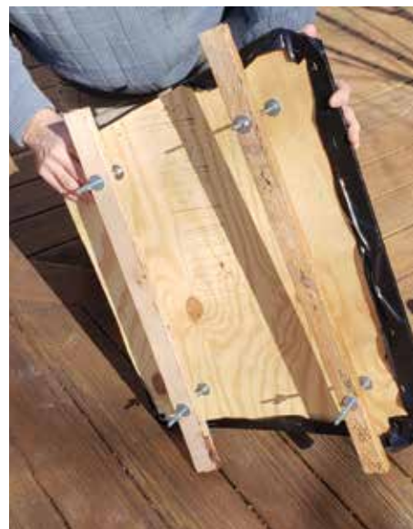
A view of the underside of the temporary hatchcover and the two attachment bars and bolts used to hold the temporary hatch in place below the foredeck.
