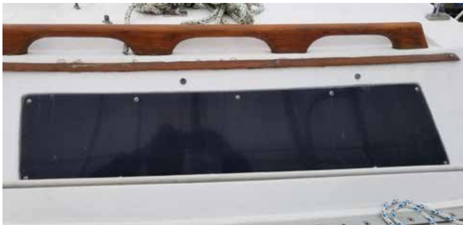
Original 30 year old windows on Afternoon delight, leaking and crazed
