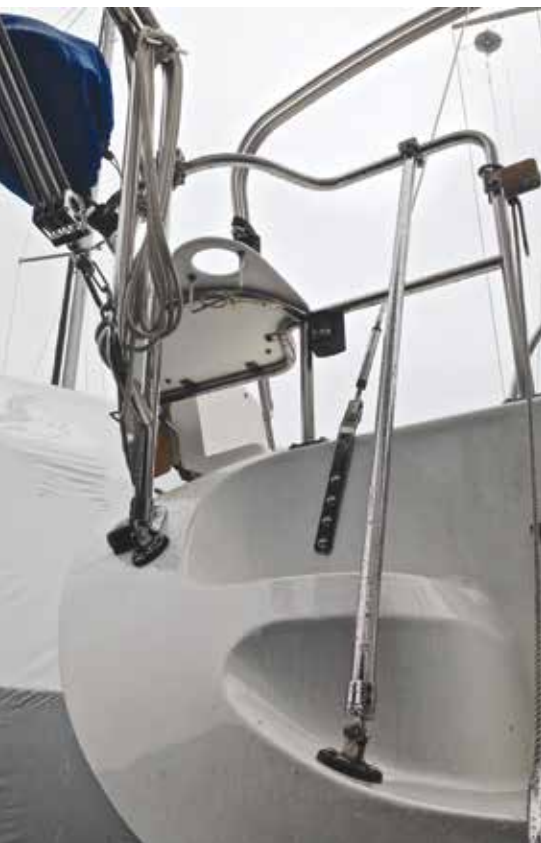
2002 C36 MKII transom design showing placement of compression strut
