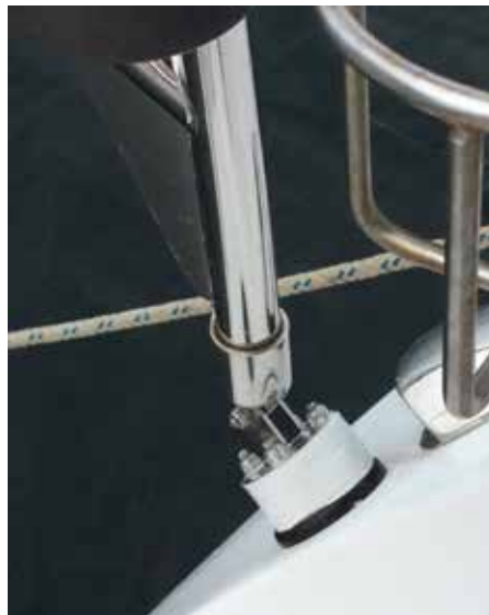
Fabricated Davit Base Spacer (wrapped with rigging tape)
