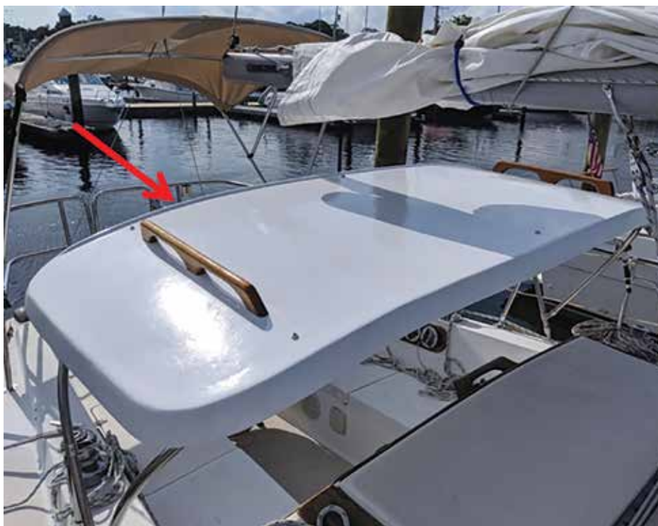
End Result. Red arrow indicates the rain guard.
