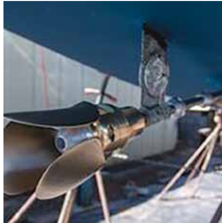
Bearing press in place and ready to go to work. Note the new cutlass bearing on the aft end of the shaft to help align the press and make sure the pressure is even.
