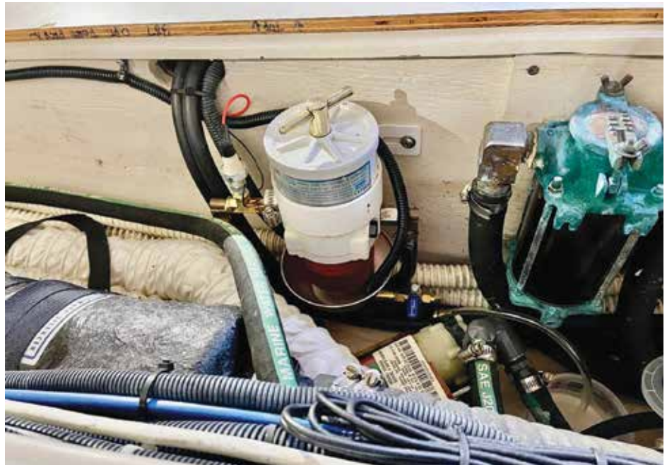
(Left) Drain valve and catch tub. (Above) Racor assembly installation.
