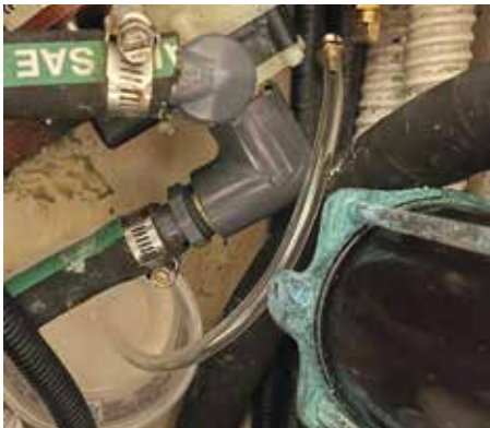
(Left) Drain valve and catch tub. (Above) Racor assembly installation.
