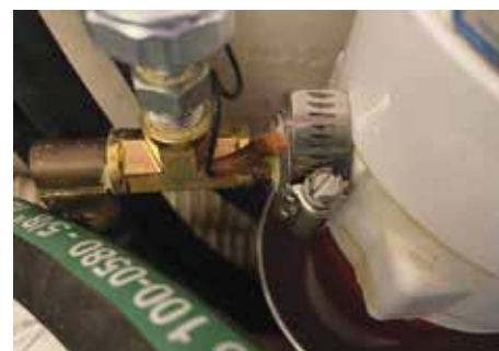
Ground wire and pressure sensor placement
