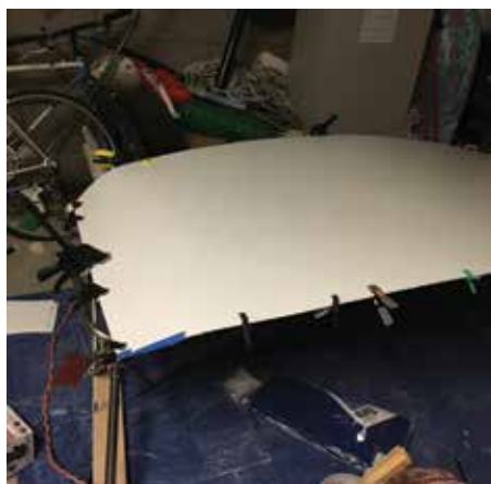
Clamped for laminating
