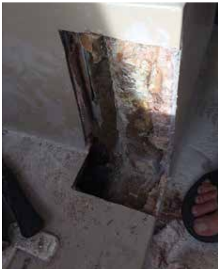
Cutting Away Corner of Dinette Seat to Access Aft Edge of Keel Trunk
