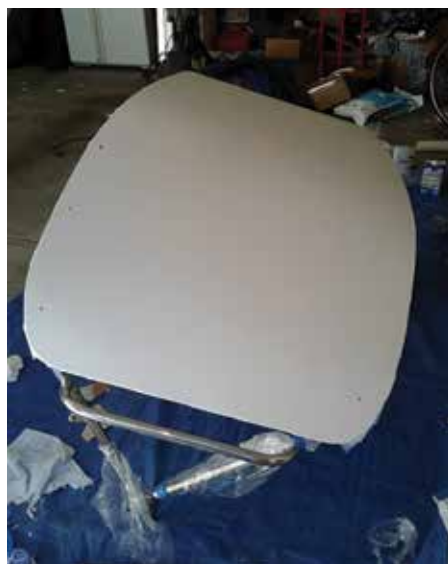
Laminated panels after the finish cut. Mounting to the Frame
