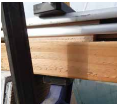
Old extrusion over new with spacer blocks
