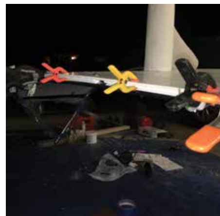
Track clamped and screwed after applying adhesive
