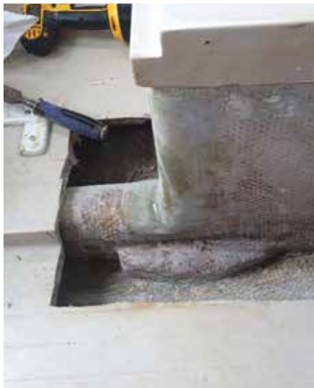
Cutting Away Corner of Dinette Seat, and Floor, for Better Access
