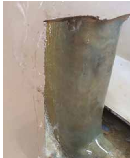
Aft Edge of Keel Trunk After Initial Fiberglass Work
