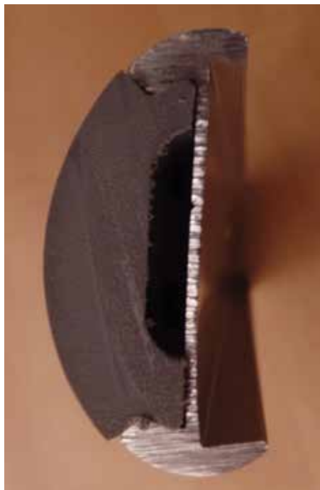
Cross-section of extrusion and insert
