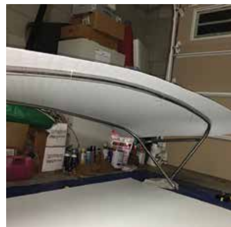
Single sheet of FRP secured to frame with wire.
