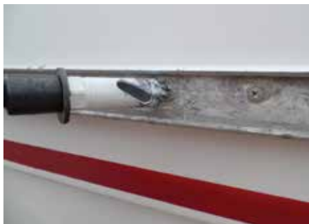
Drilling around head of machine screw
