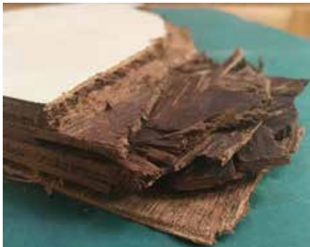
Section of delaminated bulkhead. The plywood has lost all structural integrity.
