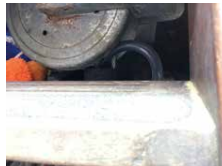
DIY Arid/Dry Bilge Pump Discharge Through Swing Keel Lifting Hardware Through-hull
