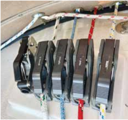
Another view. Note: clutch is sitting that far forward because I installed the baseplate backwards!
