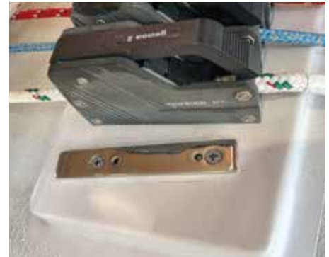
Adaptor plate installed, re-using the original clam cleat screws
