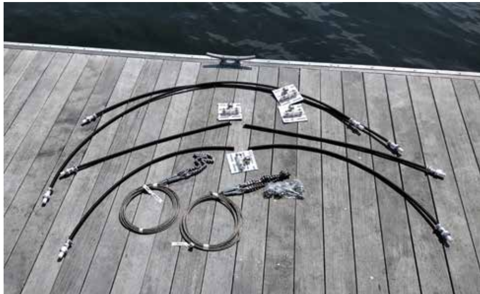
Complete kit, showing two sections cut for grease fitting insertion
