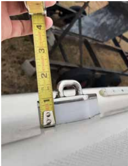
Padeye for turning block
