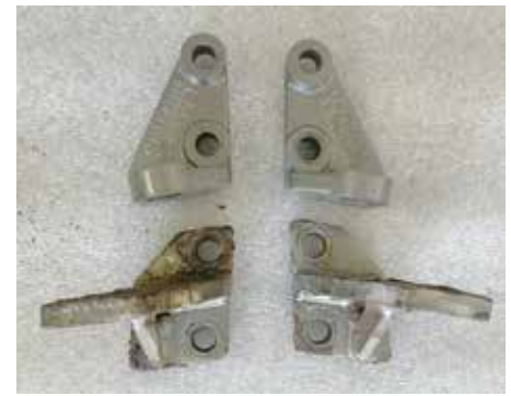
Yanmar (upper) vs Catalina custom (lower) rear engine brackets
