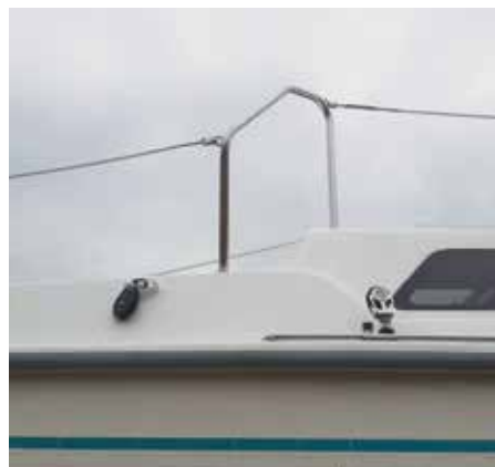
New T-Track and turning block
