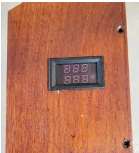
The panel removed and with the display installed - pre refinishing
