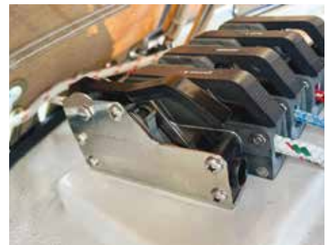
Garhauer clutch with adaptor plate installed
