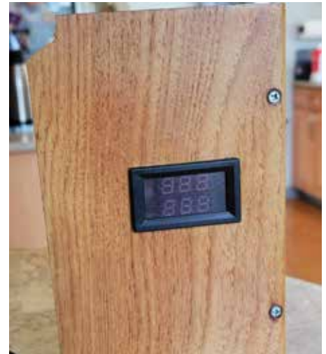
Display in the sanded panel prior to varnish and reinstall
