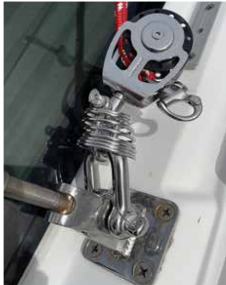
D Shackle and Block Install
