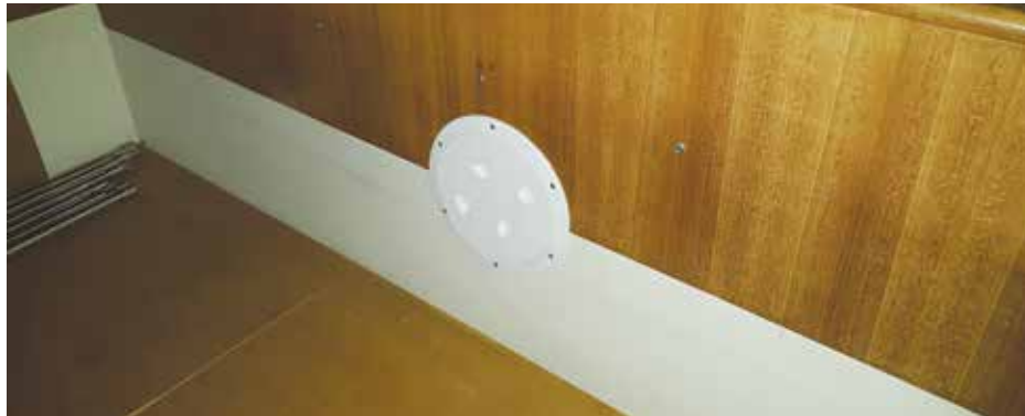
Galley Sink Access Port
