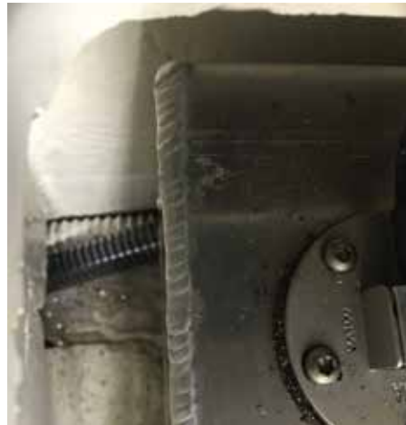
Bilge hose passing fuel tank and through bulkhead forward of the tank
