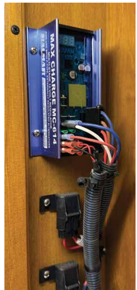
Balmar's MC-614 (now bluetooth capable MC-618) controls works with the Balmar XT alternator to safely charge the Lithium battery bank with high amperage without overheating the alternator.
