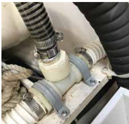
Electric bilge pump hose connection to manual bilge pump hose
