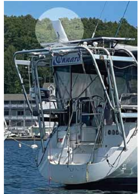
Starlink antenna mounted on Onward's stern arch.
