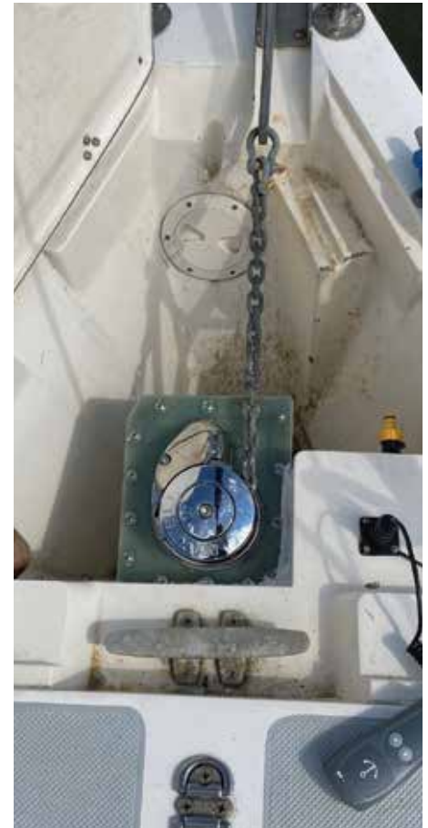
Windlass installation complete
