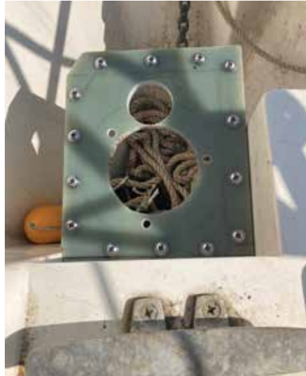
Windlass platform installed
