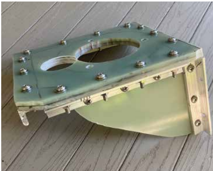
Windlass platform, side view
