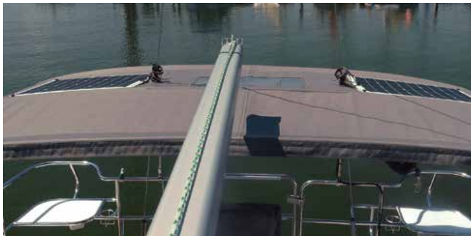
Solar panels attached on bimini attached with magnets and tied to backstays
