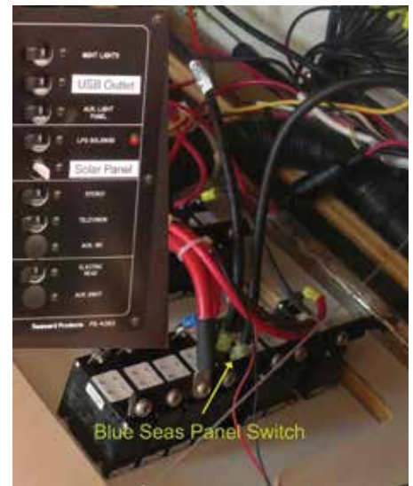
The positive solar wire was cut and attached to the switch.
