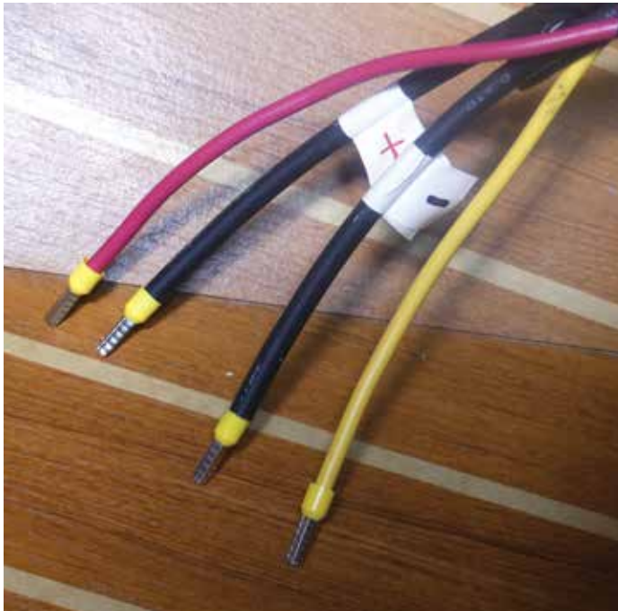
These are wire ferrules crimped on the wire ends.
